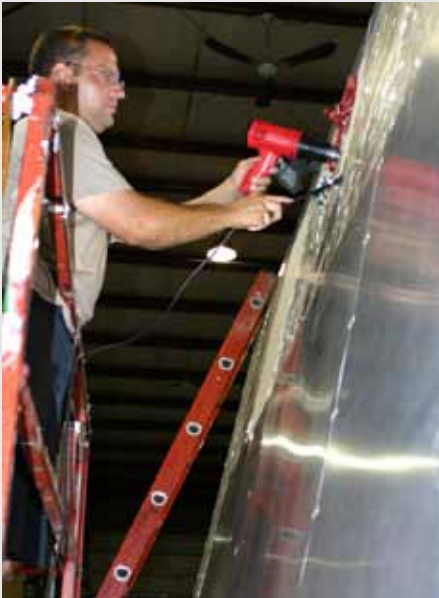
Brad White on scaffold scraping old vinyl graphics from SignTruck
